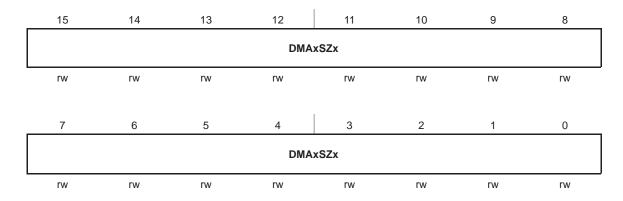
DMAxSZx Bits 15–0 DMA size. The DMA size register defines the number of byte/word data per block transfer. DMAxSZ register decrements with each word or byte transfer. When DMAxSZ decrements to 0, it is immediately and automatically reloaded with its previously initialized value.
